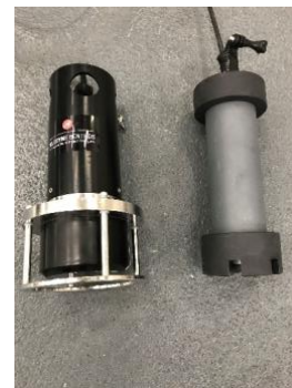
Acoustic transducer (left) transmitting acoustic commands to be received on the hydrophone (right).
