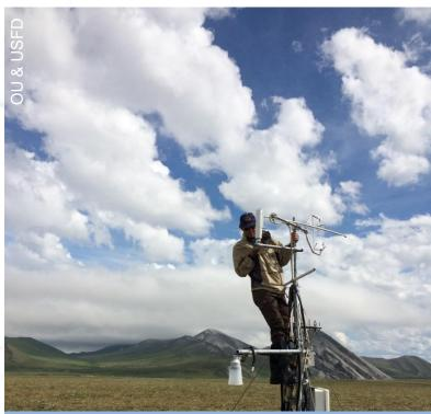
Eddy covariance tower in Ivotuk (Alaska), measuring the emission and sequestration of the greenhouse gases  $CO_2$  and  $CH_4$  from arctic tundra in summer 2016
