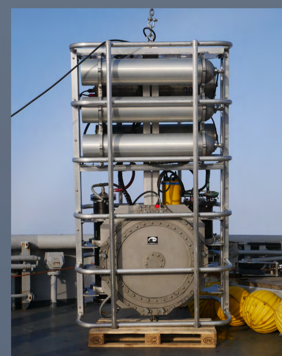
An ultra-low frequency source ( f_0 = 35 Hz, \Delta f = 4 Hz) developed by GeoSpectrum Technology Inc. The source is on the Norwegian ice breaker KV Svalbard during the 2019–2020 Coordinated Acoustic Thermometry Experiment (CAATEX) conducted jointly by the USA and Norway. The source transducer mounted in the bottom of the frame is approximately 1 m in diameter and 0.2 m thick. Above it are high pressure gas bottles for the pressure-compensation system. (Photo: E. Storheim.)
