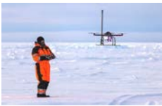
UAV with met sensors (M. Jonassen, FMI)
