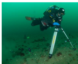
Ecological monitoring using passive acoustics deployed on the seafloor in Young Sound, Greenland. (Ref. CNRS-IUEM)
