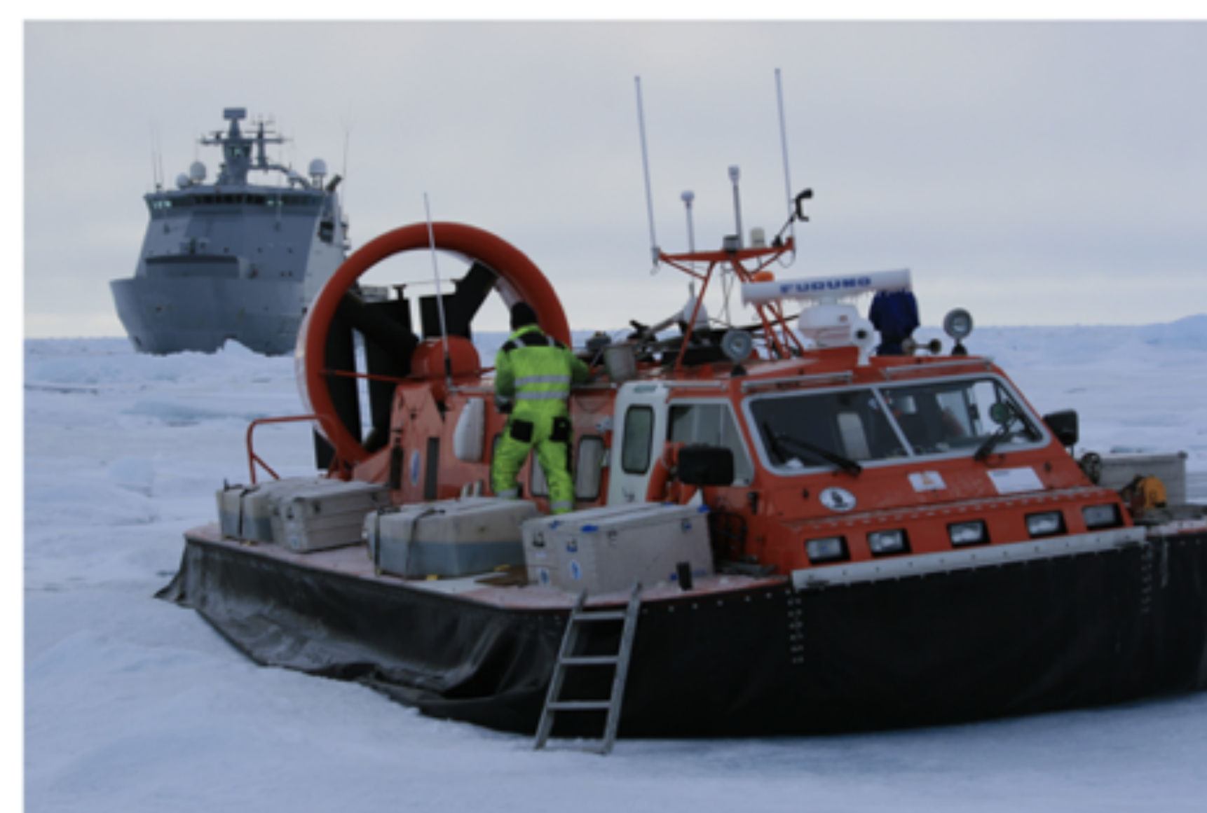
The GTI low-frequency sound source will be deployed and operated from a hovercraft. The sound-source will be deployed through an ice-hole next to the hovercraft.
