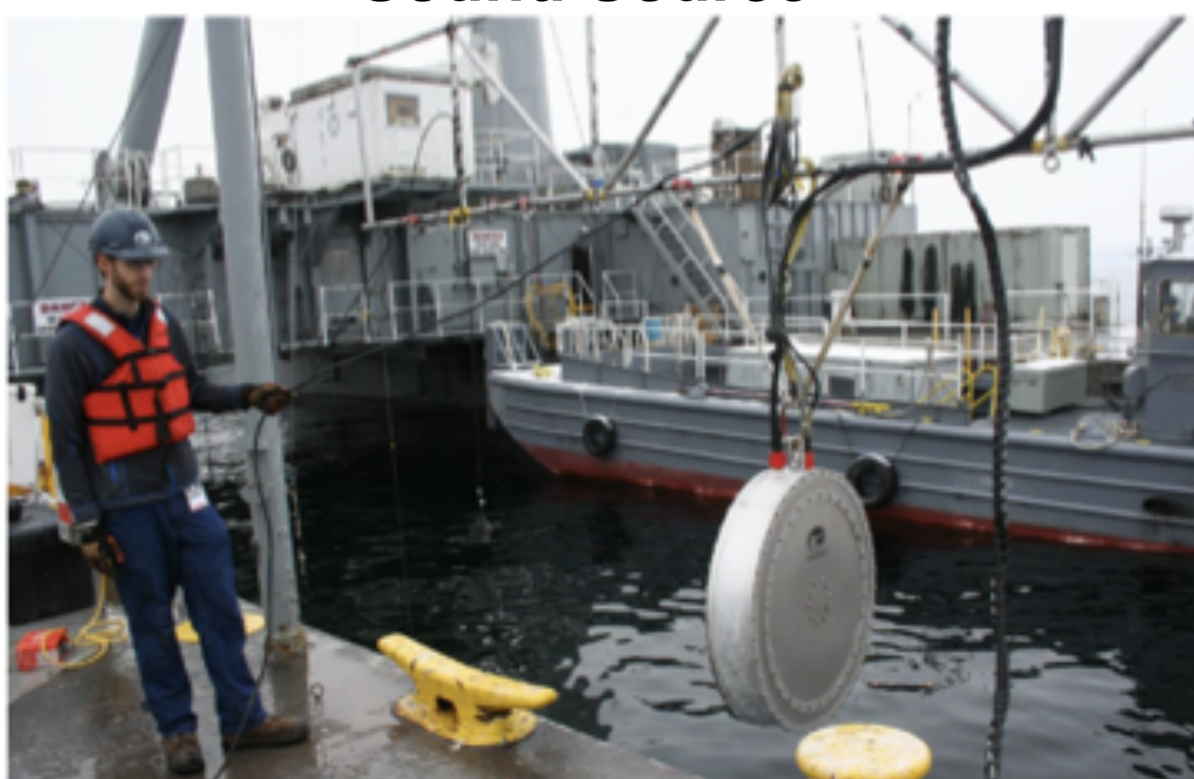
The GTI low-frequency sound source under test at the Seneca Lake Facility.
