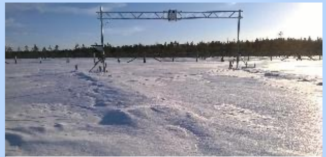
Figure 1. Deployment of spectro-albedometer in the field
