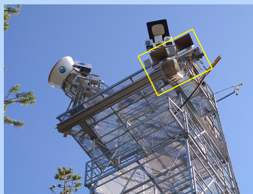
Figure 1. SodSAR mounted on a 21 m tall tower
