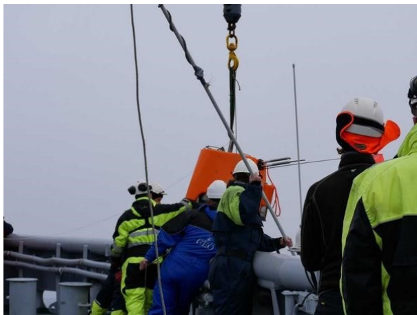
Figure 2. The orange OBS is recovered from the ocean floor after almost one year of autonomously measuring seismic and acoustic signals traveling through the earth and ocean.
