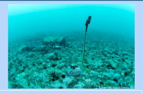
Figure 1. Acoustic recorder deployed by divers at 10m depth close to Kongsfjordneset point.
