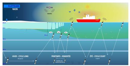
Figure 1. Illustration of bio-Argo buoys operating in partly ice-covered ocean in Baffin Bay
