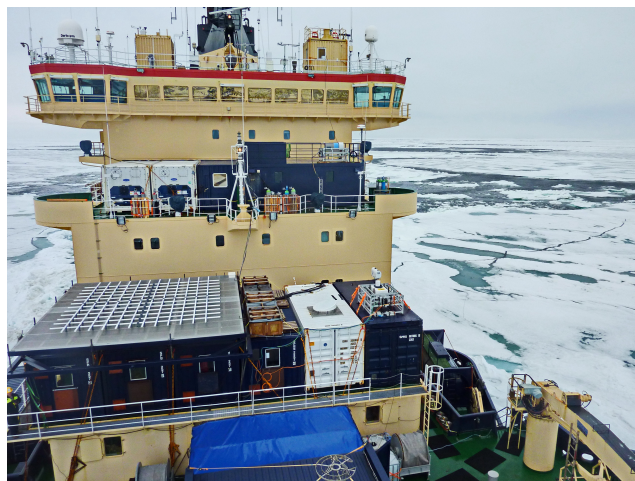
Figure 2: The observing systems are mounted in different places onboard icebreaker Oden
