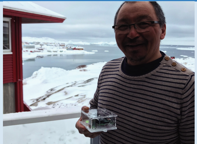
Fig. 1 Gerth Nielsen, Akunnaaq, with seismograph before connecting it to electricity and a router and placing it on the rock below his house. Photo: F. Danielsen.
