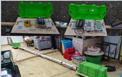
Fig. 1 The radar system consists of a transmitter, a receiver and a control unit that also includes the digital recording system, together with transmitting and receiving antennas.
