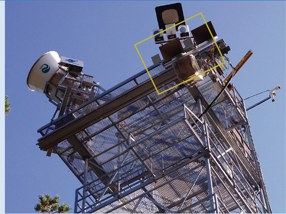
Fig. 1 SodSAR mounted on a 21 m tall tower
