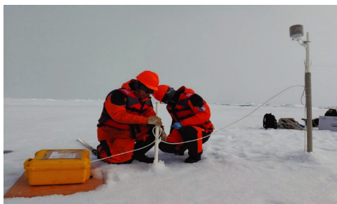
Fig. 2 Deployment of a SIMBA buoy
