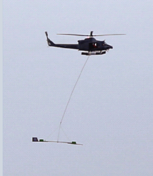
Fig. 2 Operating the radar system from a helicopter.
