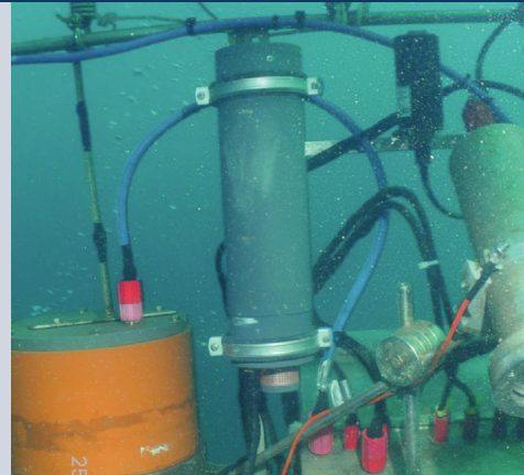
Fig. 1 Some of the instruments, including the pH sensor, mounted on the profiling platform (0 to 11 m).
