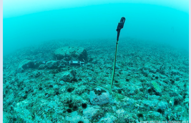
Fig. 1 Acoustic recorder deployed by divers at 10m depth close to Kongsfjordneset point.
