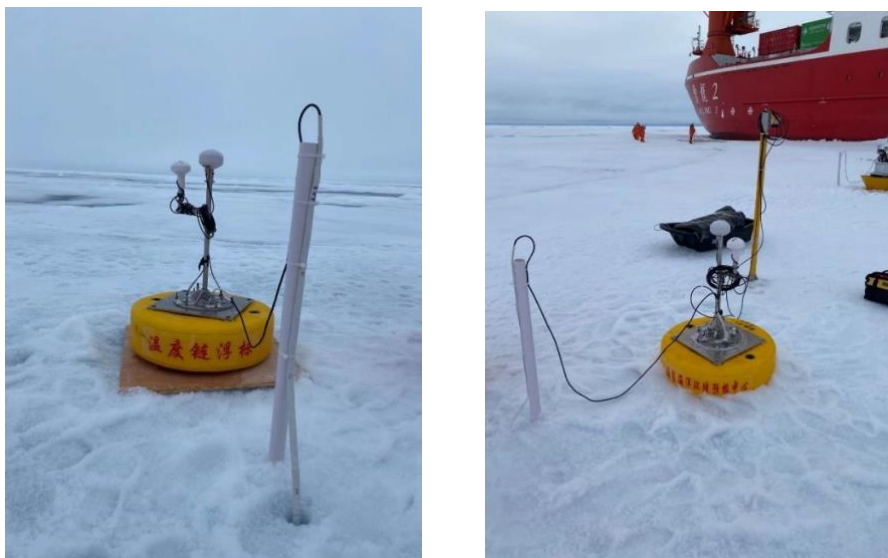
Figure 4. The UIS ice units were deployed during CHINARE2021 Arctic bathymetry survey expedition. The UIS as well as SIMBAs were deployed along the Gakkel ridge in the Arctic basin between 9 - 20 September. The ice thickness along the UIS sites were between 1.1 m and 2.2 m, the snow thickness ranged between 0.05 m - 0.1 m comparable to the values at CHARCORDry test cruise deployment sites. Photo by Zhongxiang Tian from NMEFC.
