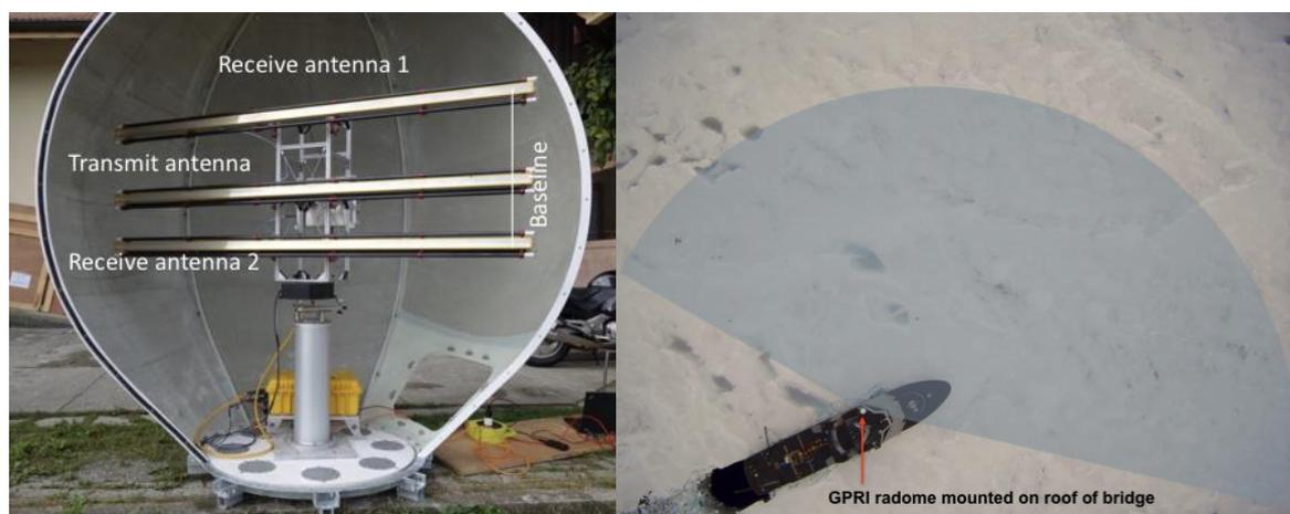
**Figure 2.** Left: The GPRI radar system consists of three rotating antennas, mounted inside a protective radome. The spatial baseline between the antennas provide sensitivity to topography. Right: The radome was mounted on the bridge roof on the forward port side. The shaded field shows the field of view of the radar. Note that the radar operated up to a distance of ca. 4 km in range.
