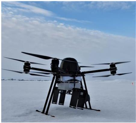
Figure 3. UWiBaSS mounted under CryoCopter FOX
