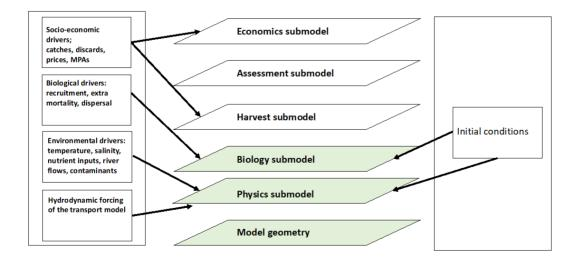
Figure 5. Modules in Atlantis. Light green is always turned on (for functionality), whereas those in white can be turned off/on after needs. NoBa has been run with the three green modules, in addition to the harvest sub-model. Box to the right shows where initial conditions are needed, drivers to the left.
