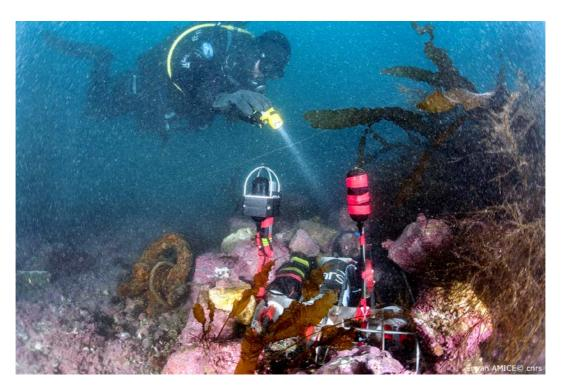
Fig. 6: Deployment of two acoustic recorders (RTSYS) at 10 m depth close to Kongsfjordneset point.
