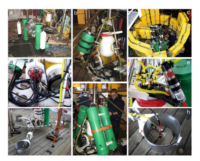
Fig. 2: Details of the arcFOCE experimental setup: a) pressure cylinders containing CO<sub>2</sub>,
