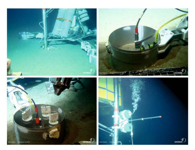
Fig. 5: Sampling of the arcFOCE experiment during RV Polarstern expedition PS121: experimental setup at 1500 m water depth in Fram Strait off Svalbard (top left), close-up of one of the mesocosms perfectly in place at the seafloor (top right), sediment sampling inside a mesocosms using ROV-handled push-corers (bottom left), blowing off excess CO<sub>2</sub> before recovering the bottom-lander (all images copyright GEOMAR).
