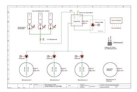
*Fig. 3: Sketch showing the main components of the experimental set-up and the control circuit of the acidification system.*
