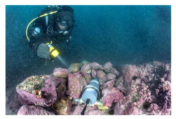
*Fig. 7: Deployment of the loggerhead LS1 acoustic recorder off Kongsfjordneset point.*
