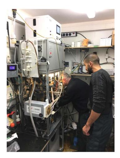
Fig. 9: Ferrybox flow-through system at AWIPEV, including a pCO<sub>2</sub>, pH, and total alkalinity (TA) sensor.
