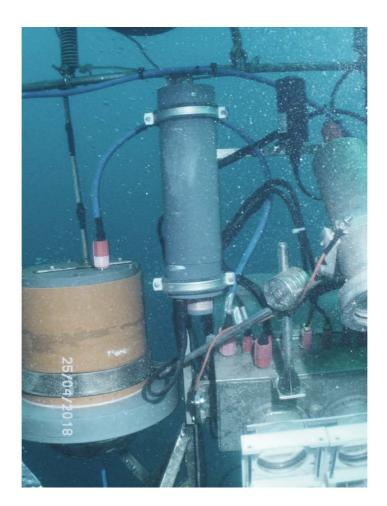
Fig. 8: Sub-sea installation in Kongsfjorden: ADCP profiler, seaFET pH sensor and a camera system (from left to right).
