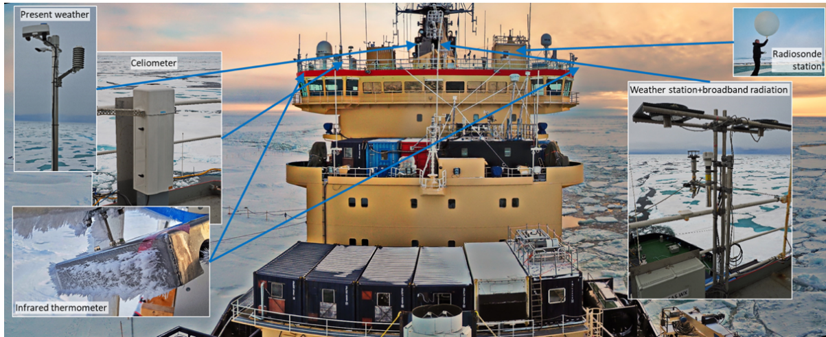
Figure 22: Front view of icebreaker Oden's superstructure indicating the locations of the instruments integrated in the advanced weather station. Left inserts show the present weather sensor, the ceilometer and the infrared thermometers for surface temperature and to the right the regular weather station with the broadband radiation sensors and the location of the radiosonde station.
