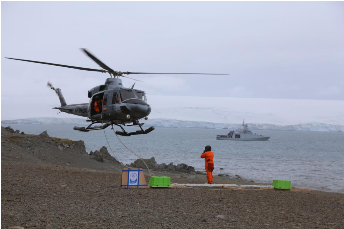
Figure 24: VIRL 20 MHz radar system mounted on a frame about to be lifted by a Bell 412 helicopter.
