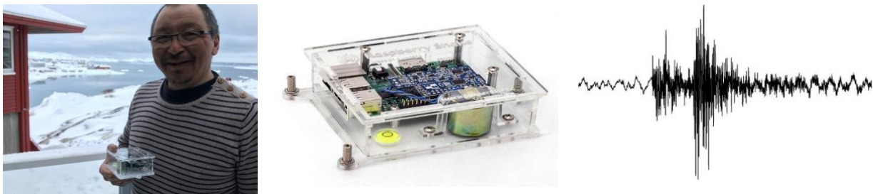
Figure 4.4. Gerth Olsen, Akunnaaq (left) with the seismometer (middle) before placing it on the rock below his house (D4.3). Photo: F. Danielsen. Right: a seismogram showing the recording of a magnitude 2.0 earthquake located 122 km South-West of Akunnaaq on 21 May 2018.
