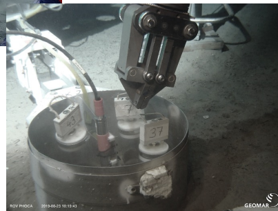
Sediment sampling before recovery in summer 2019 using ROV PHOCA
