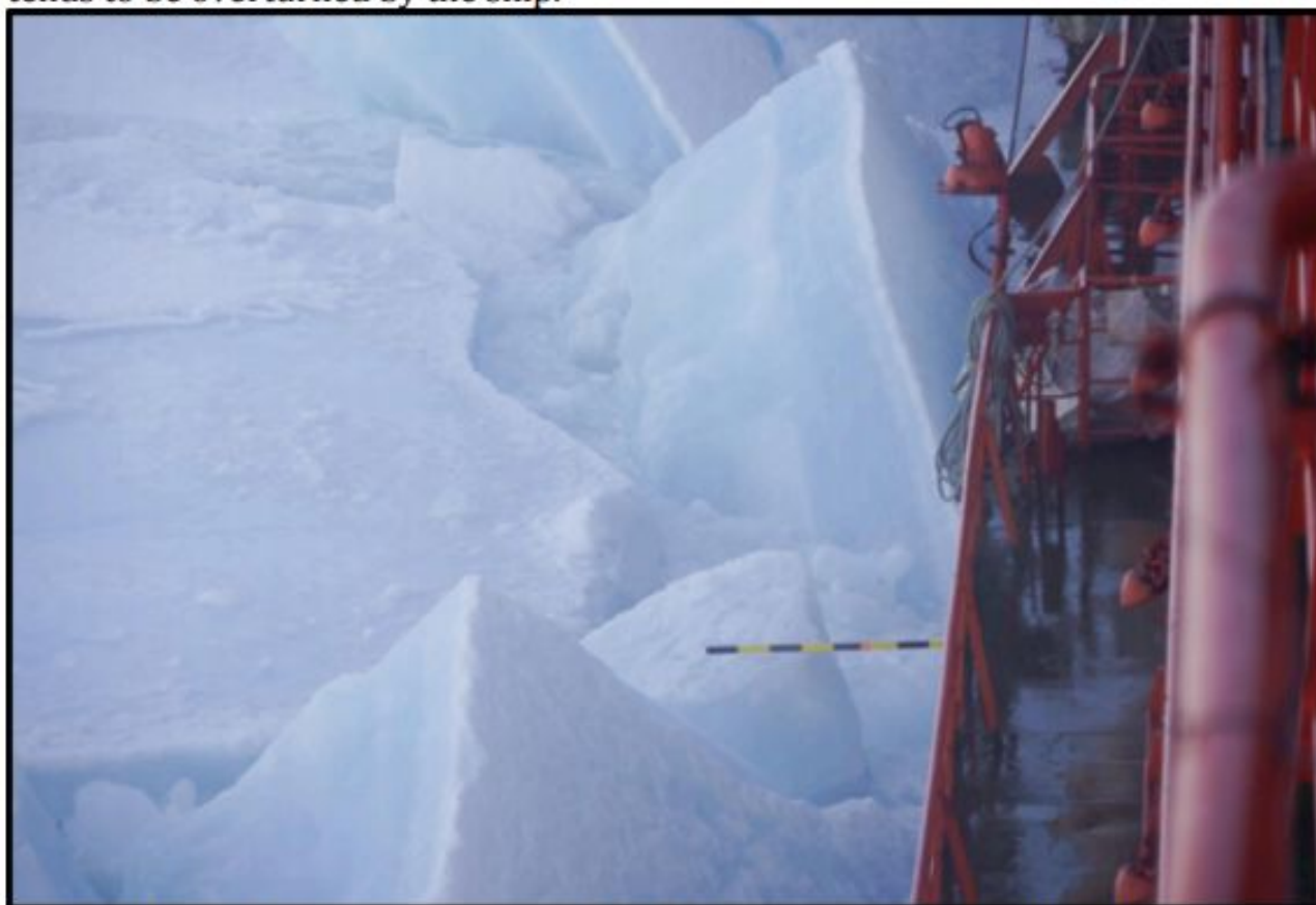
Figure 5: Painted pole used to aid eye in estimating ice thickness. Thanks Lauren Farmer and Alex Cowen.
