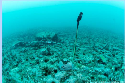
Figure 1. Acoustic recorder deployed by divers at 10m depth close to Kongsfjordneset point.
