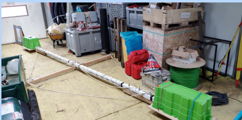
Figure 1. The radar system consists of a transmitter, a receiver and a control unit that also includes the digital recording system, together with transmitting and receiving antennas
