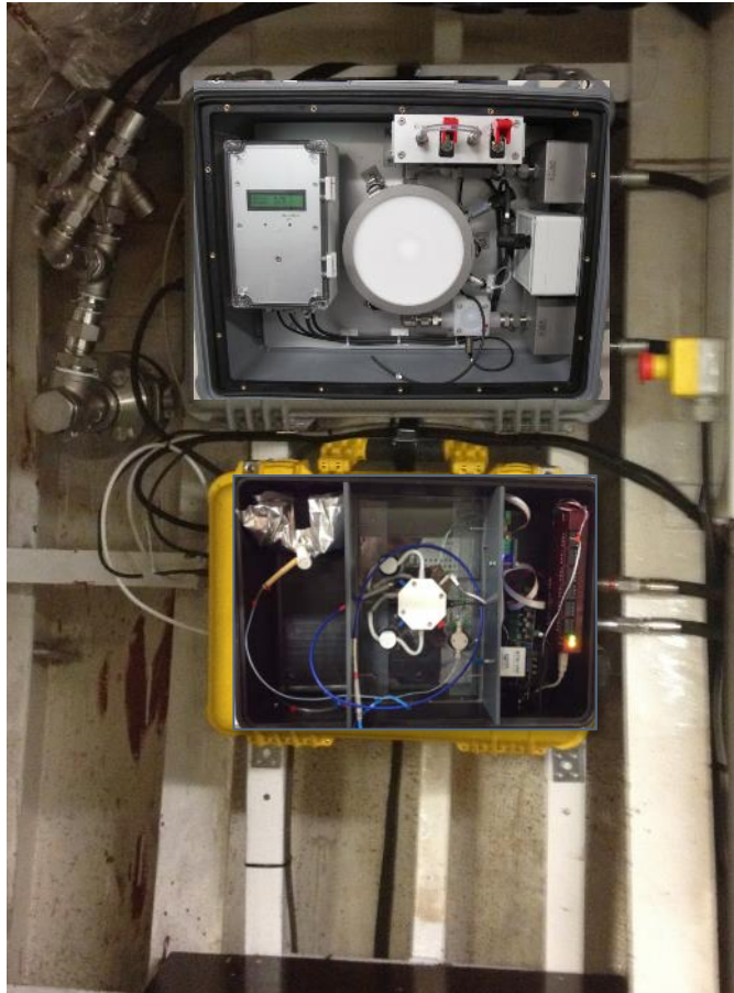
pCO 2 (top) and pH (bottom) sensors
