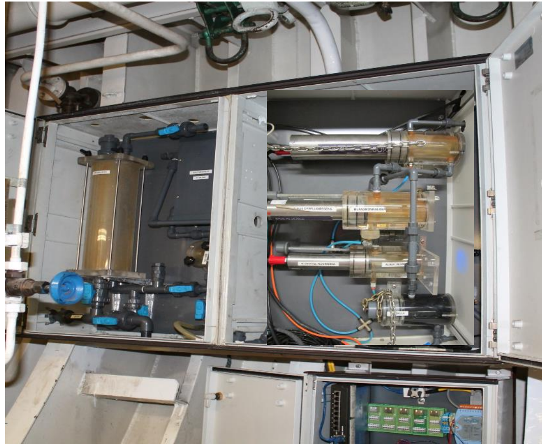
Debubbler (left) and CTD, chl a, and turbidity sensors (right)
