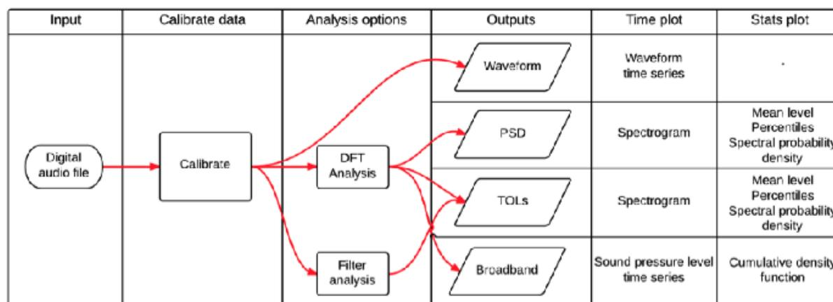
Figure 7. Data flow in PAMGuide (from supplement to Merchant *et al.* (2015)). DFT = discrete Fourier transform; PSD = power spectral density; TOL = 1/3-octave band level.
