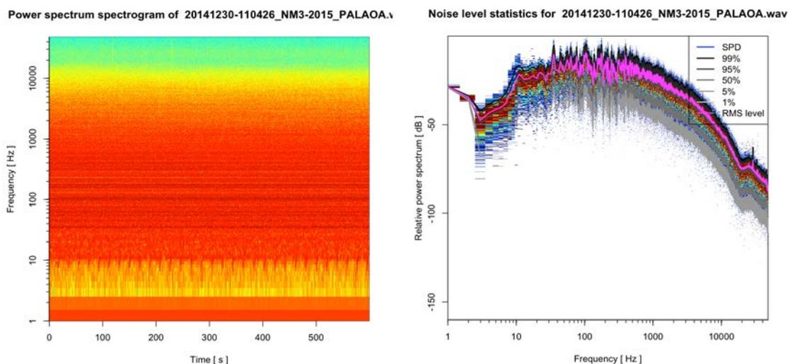
Figure 6. Examples of power spectrum spectrogram (left) and noise statistics plot (right) generated by the C-PAD Service when analysing passive acoustic data from the PALAOA observatory in Antarctica (<https://doi.pangaea.de/10.1594/PANGAEA.773610>).
