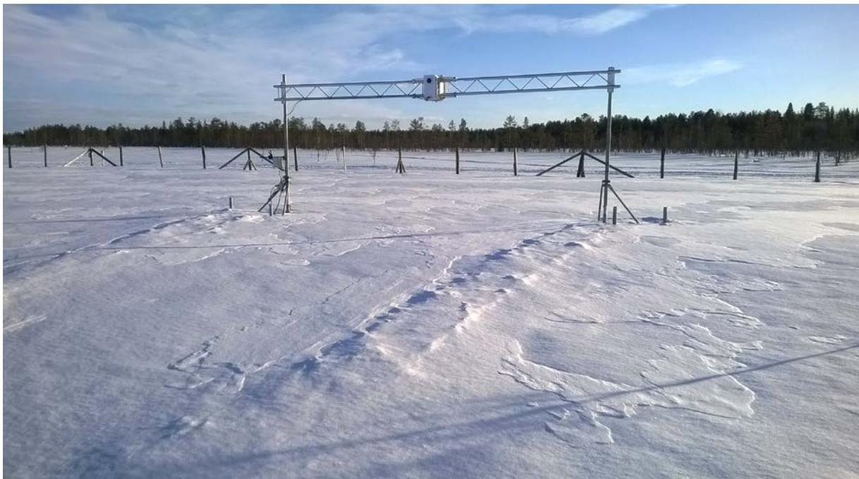
*Figure 7: SVC-FMI spectro-albedometer installed in Sodankylä, Finnish Lapland.*
