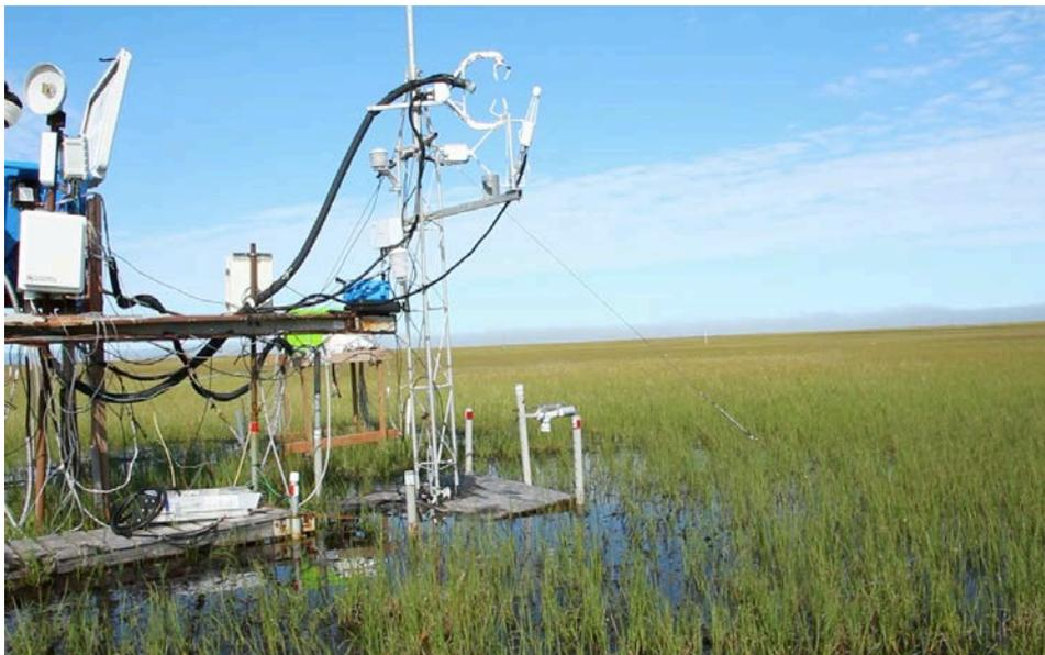
*Figure 5. New heated sonic anemometer installed in Barrow Alaska during summer 2019.*
