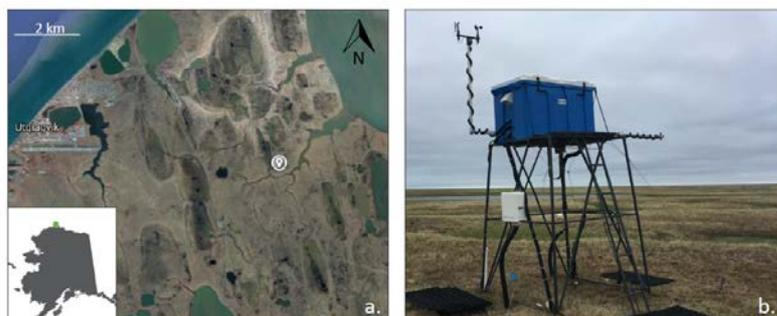
Figure 4. (a) Location of the study relative to Barrow (AK); (B) Sub-surface CO<sub>2</sub> and CH<sub>4</sub> monitoring system with associated meteorological measurements.
