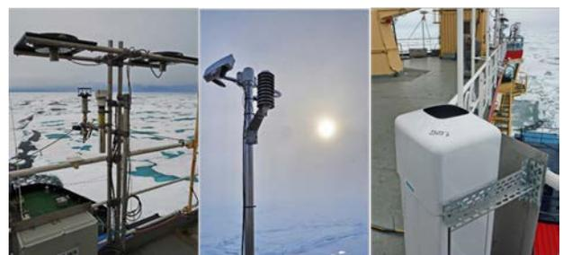
Figure 11. Photos of instruments deployed on the 7<sup>th</sup> top deck (“monkey island”) showing (left) the weather station with the two long- and shortwave broad band radiation sensors in their gimbals, (middle) the present weather/visibility sensor and (right) the ceilometer lidar. All are along the forward railing. Not shown are two infrared thermometers, one on each side looking down at the surface; surface temperature facilitates calculation of upward longwave radiation.
