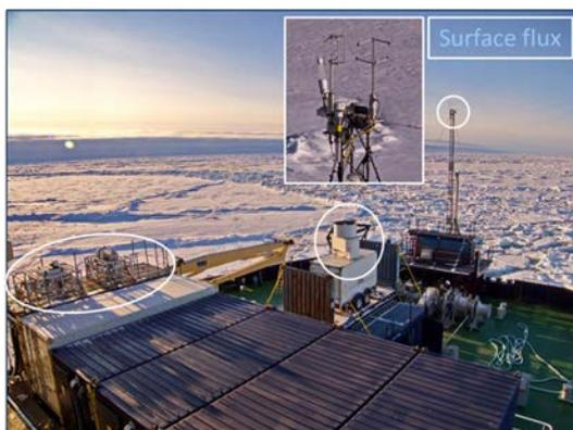
Figure 10. Photo of the foredeck installations with the foredeck mast with sonic anemometers and gas analyzers for surface flux observations. Also in this photo are the Doppler cloud radar, lidar and the scanning microwave radiometer that was deployed in AO2018 by collaborating groups.
