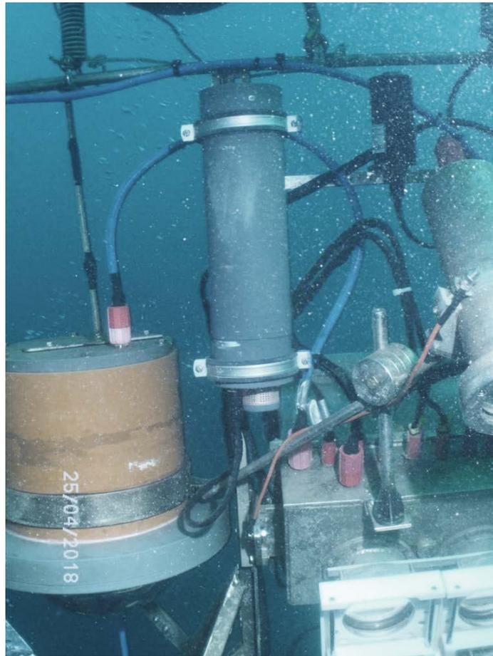
*Fig. 8: Sub-sea installation in Kongsfjorden: ADCP profiler, seaFET pH sensor and a camera system (from left to right).*
