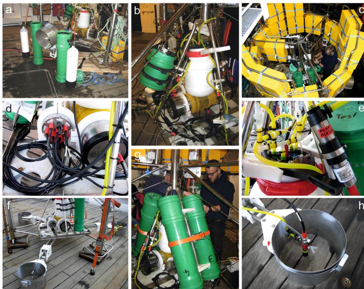
*Fig. 2: Details of the arcFOCE experimental setup: a) pressure cylinders containing CO<sub>2</sub>, b) in-situ calibration unit (green) and mixing container (white), c) ring of syntactic foam bricks of the bottom-lander system, d) control unit and battery housing, e) pumps delivering acidified seawater to the mesocosms, f) lander frame carrying a total of three mesocosms, g) tubes housing the pressure cylinders, and h) pH sensor in one of the mesocosms.*
