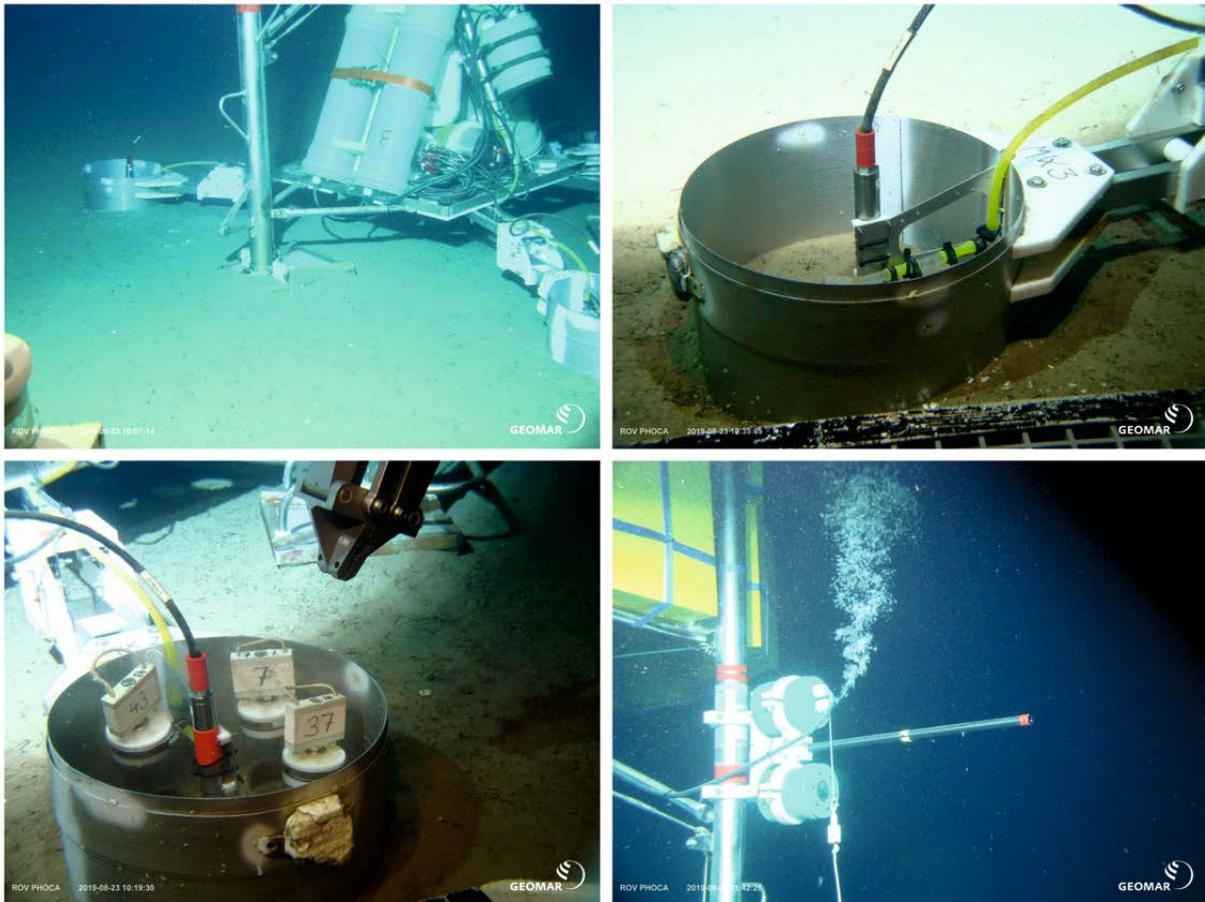
*Fig. 5: Sampling of the arcFOCE experiment during RV Polarstern expedition PS121: experimental setup at 1500 m water depth in Fram Strait off Svalbard (top left), close-up of one of the mesocosms perfectly in place at the seafloor (top right), sediment sampling inside a mesocosms using ROV-handled push-corers (bottom left), blowing off excess CO<sub>2</sub> before recovering the bottom-lander (all images copyright GEOMAR).*
