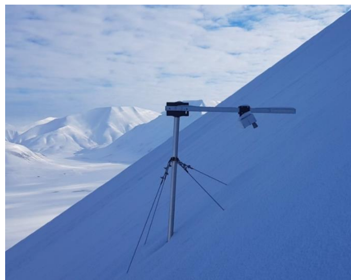
Figure 10 (a) Manually observed snow avalanches in Longyearbyen area in Svalbard. The numbers are observed incidents registered in www.regobs.no ; (b) An automatic snow observation station in a release area near Longyearbyen (Photo: Martin Indreiten). (Engeset et al., 2020)
